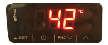
SET Press set button until **UnL** (Un lock) is shown in the display.
